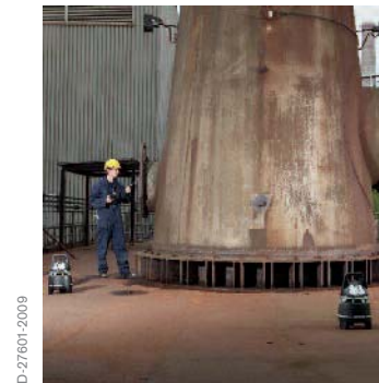
Wireless fenceline Up to 25 Dräger X-zone 5000 automatically interconnect to form a wireless fenceline.
