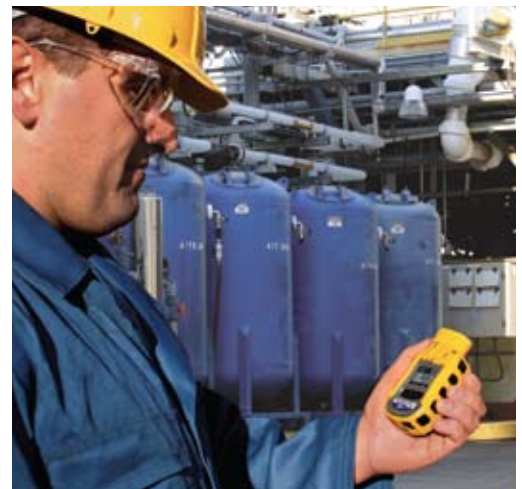
Worker exposure monitoring with ToxiRAE Pro PID
