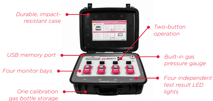
PROTÉGÉ ZM TEST STATION
