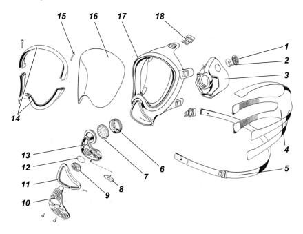
Fig. 3 Full face mask exploded view
