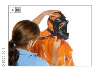
Evenly pull the straps of the mask towards the back. The sealing lip of the mask must rest on the facial cuff, not on the suit material or seam.
