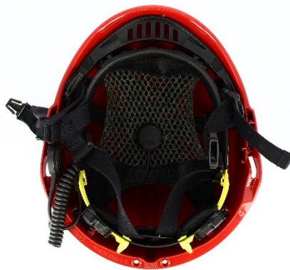
Bone conductive sensor mounted inside helmet
