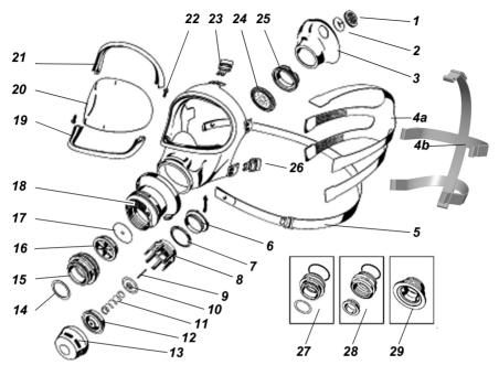
Fig. 4 Full face mask exploded view
