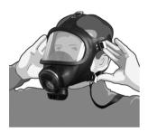
(1) Loosen the head harness, press the buckles forwards using your thumbs.
