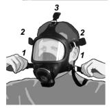
(4) If necessary adjust mask and tighten the straps in order as shown firmly and evenly.
