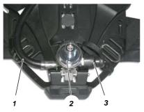
Fig. 3 Pressure reducer SingleLine
