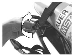
Fig. 18 Opening the cylinder buckle
