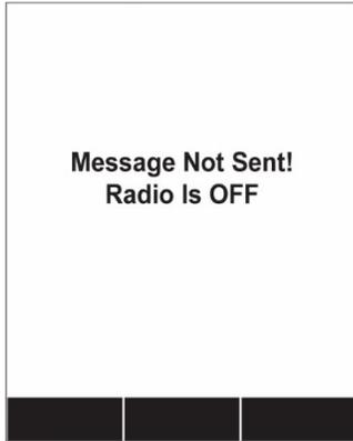
After a few seconds, the display automatically returns to the Send Message screen. Check that the radio module is turned on. If it is off, turn it on and try sending the message again.
