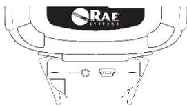
3. Press Travel Charger onto bottom of MultiRAE.
