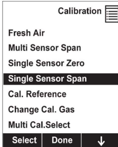
6. Press [Y/+ ] to start calibrating. You can abort the calibration at any time during the countdown by pressing [N/-].
