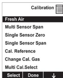
After a timer countdown, the zero calibration is done. The LCD displays the sensor names and tells you whether each calibration passed or failed, followed by the sensor readings.
