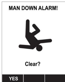
In addition, the instrument alarms (audible and visible) four times per second. The instrument also sends an emergency message to Safety Suite Device Configurator (SSDC).
