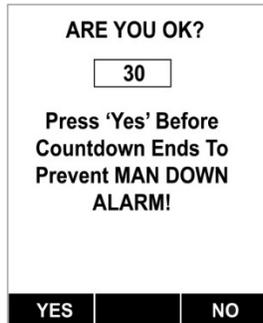
If you do not need assistance, press [Y/+] before the countdown reaches 0 to stop the Man Down alarm from being activated. Otherwise, press [N/+] to trigger the Man Down alarm immediately, or do not press either key (the countdown will reach 0 and the alarm will start). When the Man Down alarm occurs, this screen is displayed:
