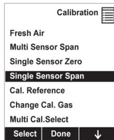
6. Press [Y/+] to start calibrating or wait for calibration to start automatically.
