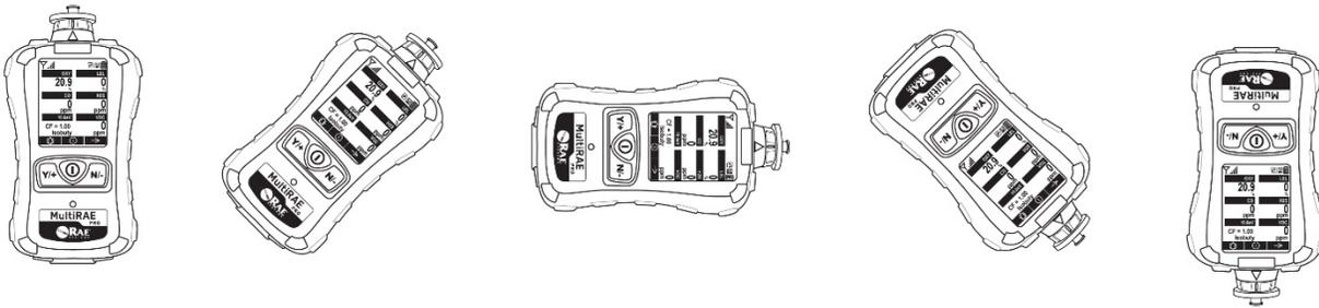
As the MultiRAE is tilted, the gravity sensor detects its orientation and inverts the screen when it is past its horizontal position.
