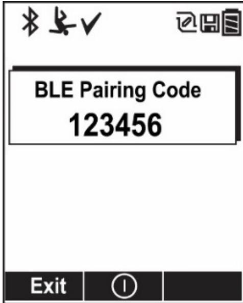
Type the pairing code into mobile app to pair the instrument and the smartphone/mobile app.
